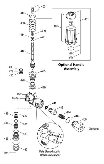
To convert to optional handle assembly, remove items 403 (quantity 2), 409 and 410. Then reassemble as shown in item 401.
